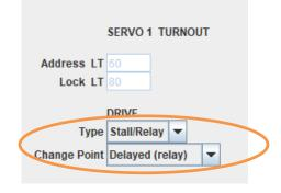
Set the **Type** to **Stall/Relay**Set the **Change Point** to **Delayed or Immediate** as desired
