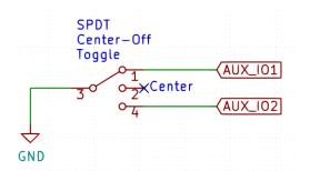
Wire the SPDT center-off toggle switch as shown in this schematic. Next configure the *QuadLN\_S*, Aux IO1 and Aux IO2 as shown below.
