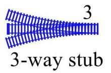
Suppose that a 3-way stub turnout is driven by Servo 3. We use **Midpoint** mode for Servo 3 so that whenever the Lock is THROWN the servo moves to the travel Midpoint, selecting the center route through the turnout. When the Lock is CLOSED the servo moves to a travel endpoint, selecting one of the diverging routes through the turnout.
