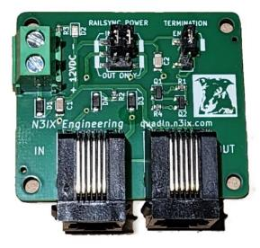
There are 2 **Jumpers** for Railsync Power Routing and 1 **Jumper** for Termination Enable.
